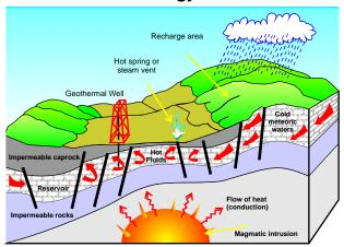
The above diagram describes the mechanism in underlying geothermal systems. Heat is supplied at the base of circulation system. Cooler recharge water from the surface of the earth's gravity feeds downwards through the earth's sub-layers and through a process of fluid convection, hot fluids rise to the upper part of the system ie entering into the groundwater table. It is estimated that shallow groundwater in Ireland has a temperature range between 9° & 12° c.
